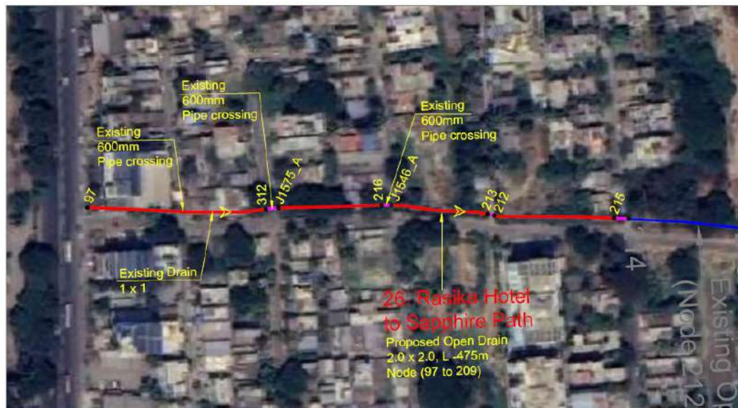
PROPOSED OPEN DRAIN (2.0 X2.0 ) OF FLOOD LOCATION AT RASIKA HOTEL TO SAPPHIRE PATH (FR OM NODE 97 TO 215)
